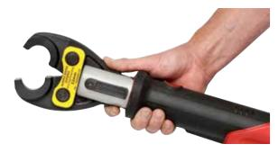
9. By squeezing the back of the jaw, the jaws will open. If you look at the machined profile on the inside of the jaws you will note a slot on each side of the profile.
