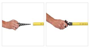
7. Insert the approved calibrating/deburring tool into the pipe, and then alternately turn in a clockwise and in a counter-clockwise direction. Ensure that a consistent, smooth chamfer is formed on the end of the pipe.
