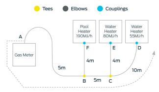
Index Run  $A \rightarrow D = 20$  metres (from the meter to the furthest appliance)
