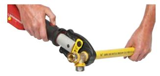
Press the switch mechanism until the joint is completed and the piston has retracted back into the body of the tool.
