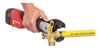
12. Press the back end of the jaws and remove the completed joint.
