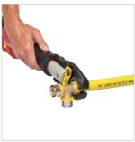
10. With the jaws open place the fitting inside the jaws so that the raised section of the plastic sight ring fits into the slot in the jaws. Release the jaws so they fit snugly over the fitting, ensuring that the raised section of the plastic sight ring is still located in the slots in the jaw.
